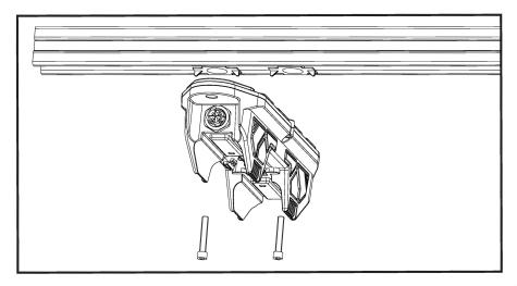
2.Attach the ThinkGrow Light Driver (TLD) to the C-channel steel using the Hex Socket Head Cap Screws.
