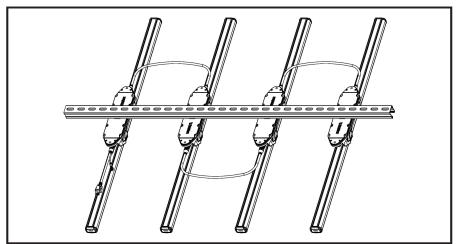
6. When the installation is completed, your LED system should look something like the image above. Ensure all connections and hardware is tight.
